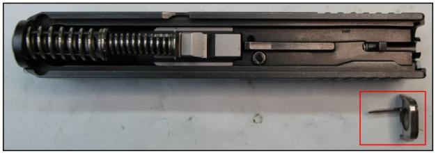
An increased danger of the defendant's version of the machinegun conversion device is that the device is flush with the stock backplate of the pistol slide. A shooter handling the defendant's machinegun would have no way of distinguishing this machinegun from a semi-automatic pistol. Thus, a shooter expecting to fire one round per trigger pull (the typical functioning of a semi-automatic firearm), instead releases an uncontrolled, fully automatic barrage of bullets.
