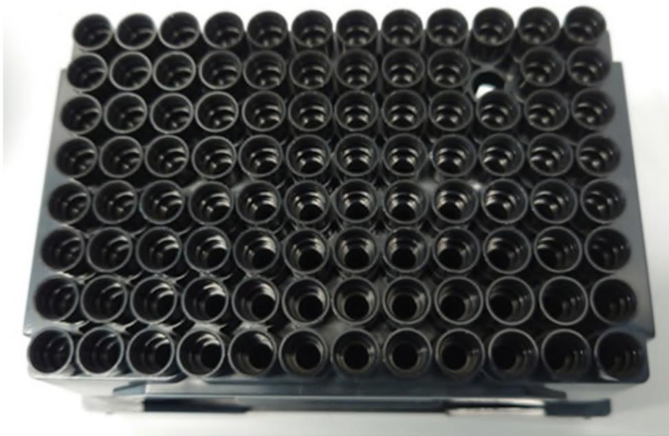
43. Ginkgo encountered similar issues with defective 1000 uL GEB Tips in its inventory. On three separate occasions involving a particular lot of 1000 uL GEB Tips, multiple tips fell off a Hamilton robot's multi-probe head, causing spillage during the liquid handling event.
